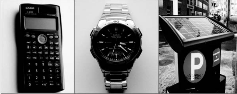
Figure 10.1 The use of solar energy in low-power and DC applications for convenience. See also Colour Insert.
